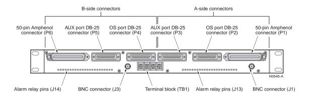
Figure 5. HRM-238 Shelf Backplane Connectors (back view)
